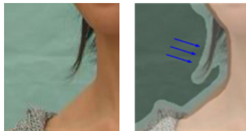
Figure 3.3: Another example that local samples are not reliable for estimation. According to different shooting angles, some hair strands are not connected with other parts. In this case, local foreground samples cannot provide true color information for mixed pixels.
