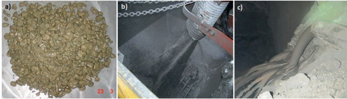
Figure 2.2 Main backfills used: (a) Rock, (b) Hydraulic, and (c) Paste backfills (Yilmaz & Guresci, 2017)
