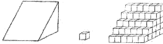
Figure 2. 8. An object and its voxel representation (reproduced from [70])
