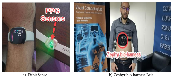
Figure 4.4: Fitbit sense and Zephyr bio-harness Belt to continuously measure Heart/Respiration and EDA metrics.
