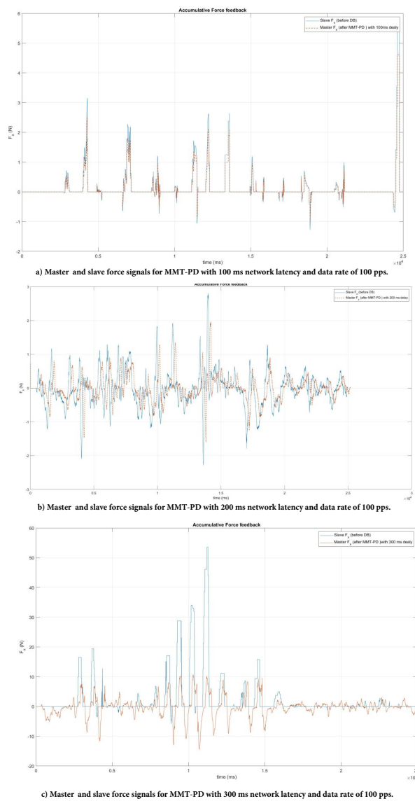
Figure 5.8: Measurements of the force signal of the master and slave during MMT+PD control scenarios.
