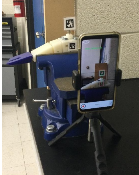
Figure 6-7: Pre-cast SLL SH sagittal testing configuration
