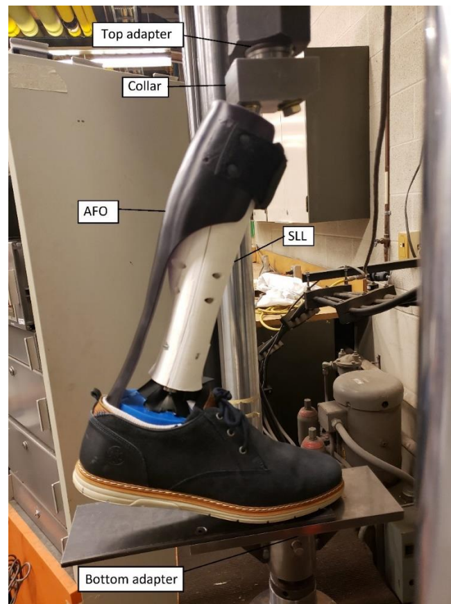
Figure 4-18: SLL on the testing apparatus in the forefoot position
