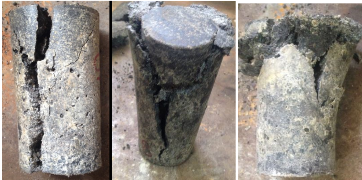
a) Longitudinal failure b) Failure with cone formation c) side fracture
