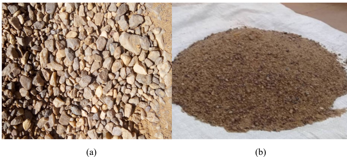
Figure 5-29: (a) Natural gravel from Niger River in Bamako, Mali and (b) image of the sand sample used in the experiment
