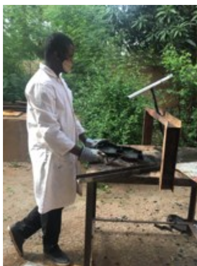
A 2-3: Conditioning the mold by injecting the lubricant, pouring of the liquid products (MPB and PWC) in the mold, compaction with the manual press
