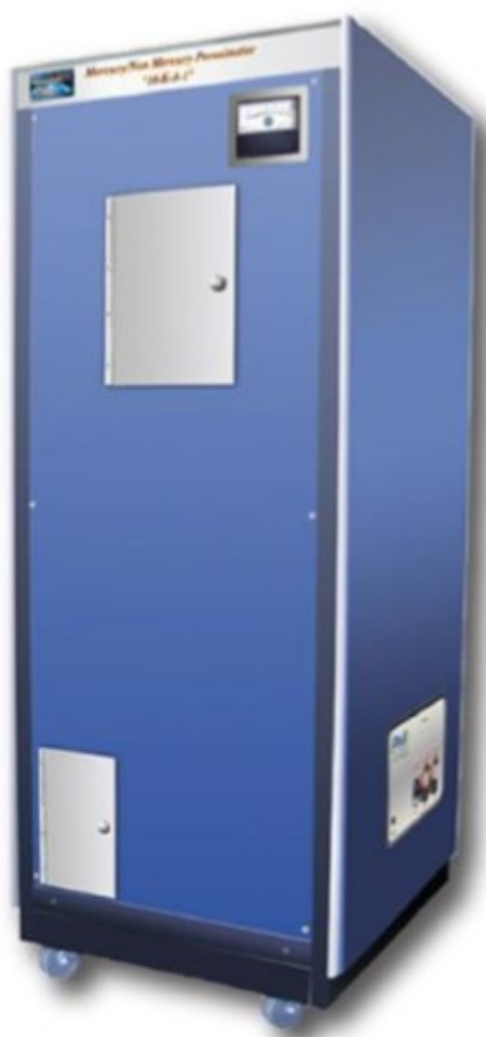
A 4-5: PMI Mercury/Nonmercury Intrusion Porosimetry instrument used to determine pore size distribution, total pore volume and surface area of the samples
