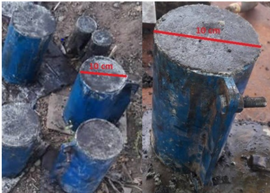
Figure 4-3: Samples of MPB before and after extraction from the mold.
