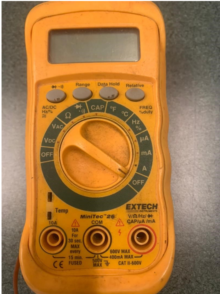
A 4-5: Multi-meter used to record temperature during the experimental program
