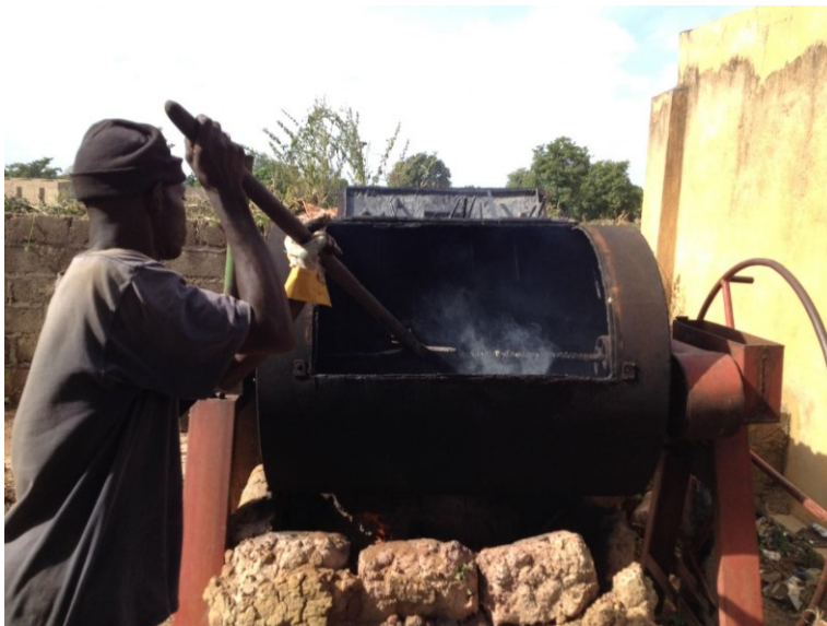
A 2-1: Melting and preparation of MPB and PWC products in the manual oven under high temperature
