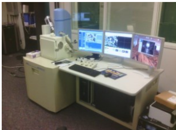
A 4-4: SEM equipment (JEOL 6610LV SEM) located in ARC building at University of Ottawa used to perform SEM analysis on samples in load cell experiments
