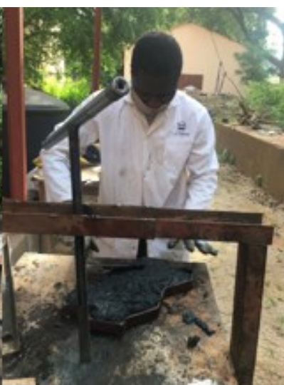
A 2-3: Conditioning the mold by injecting the lubricant, pouring of the liquid products (MPB and PWC) in the mold, compaction with the manual press
