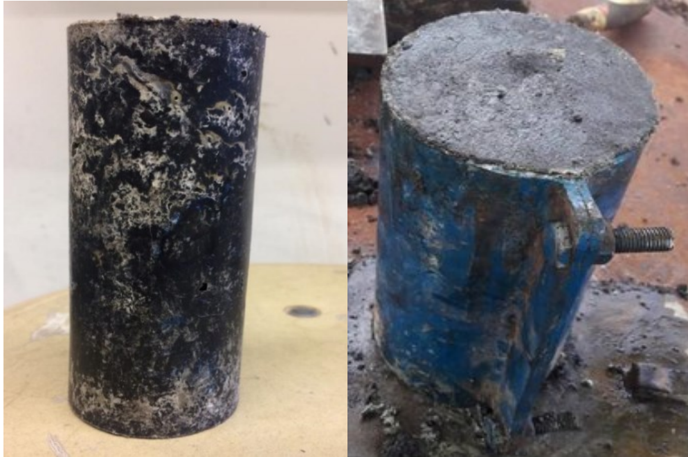
a) 5 cm in diameter and 10 cm in height b) 10 cm in diameter and 20 cm in height Figure 5-4: Samples of PWC with melted plastic wastes before (right) and after (left) demolding.
