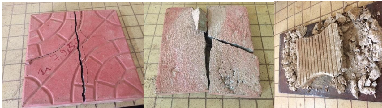
A 3-3: Some samples of pavers sold on Bamako's market (Mali, before and after compression tests)
