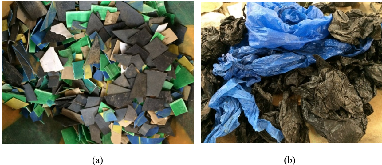
Figure 4-26: Samples of a) HDPE and b) LDPE plastic wastes used during the experiments.
