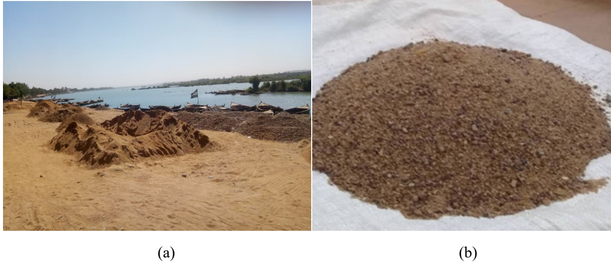
Figure 4-1: (a) Sampling site of the sand in Kalaban - Coro on the banks of the Niger River in Bamako, Mali and (b) image of the sand sample used in the experiments
