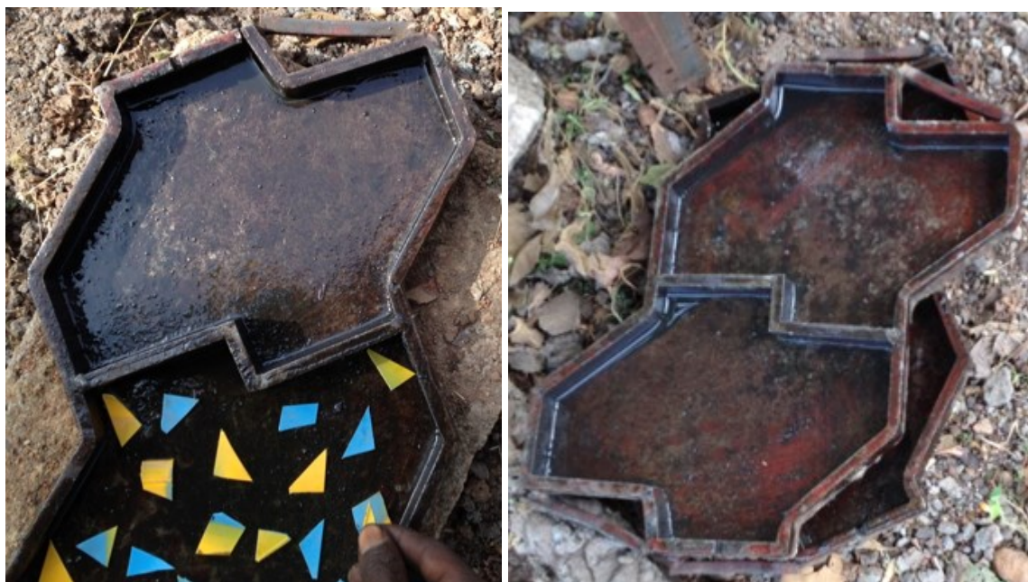
A 1-7: Molds used for the production of MPB and PWC
