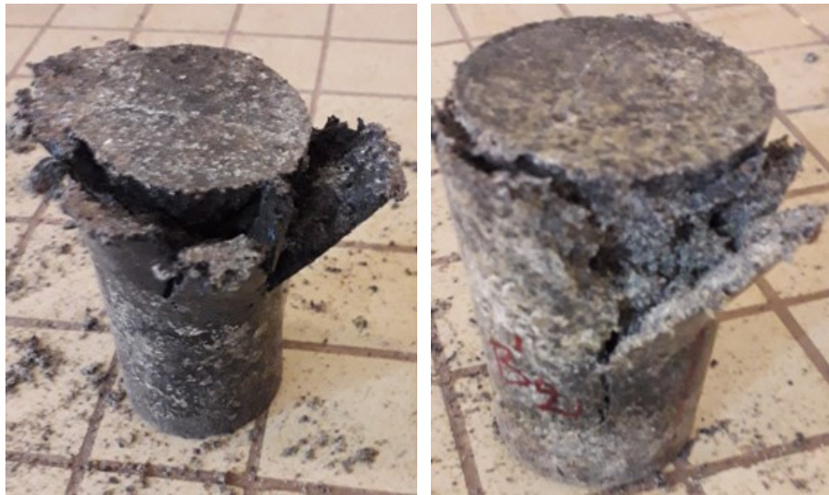
a) 50%P – H/L 50/50 samples after compressive strength tests
