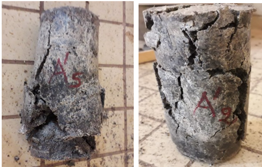
b) 50%P – H/L 60/40 specimen after compression
