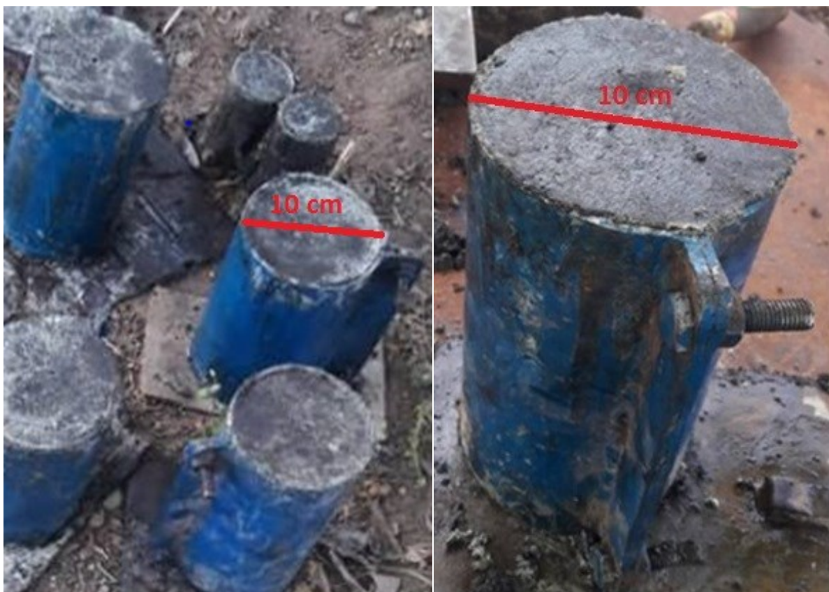
Figure 4-29: Samples of MPB with melted plastic wastes as binder before and after demolding.
