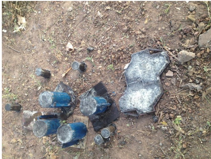
A 3-1: Prototypes of pavers using MPB (interior backyard) and PWC (bearing heavy load) made from plastic wastes before and after demolding
