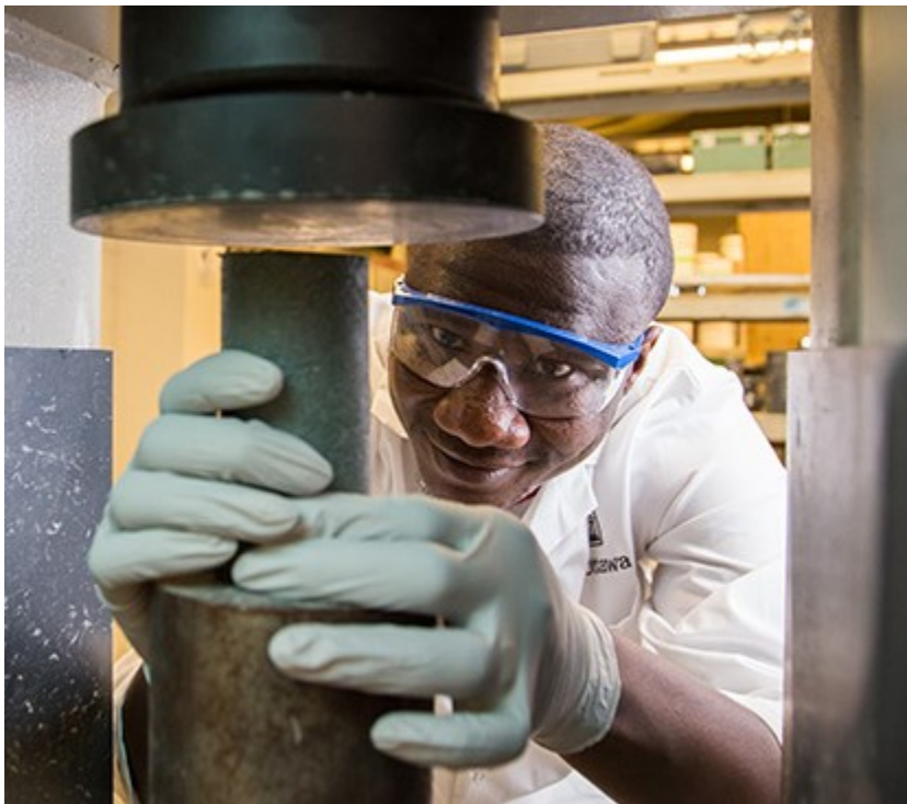
A 4-1: Performing COMPRESSIVE STRENGTH test on PWC sample
