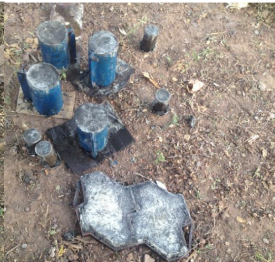
A 3-1: Prototypes of pavers using MPB (interior backyard) and PWC (bearing heavy load) made from plastic wastes before and after demolding
