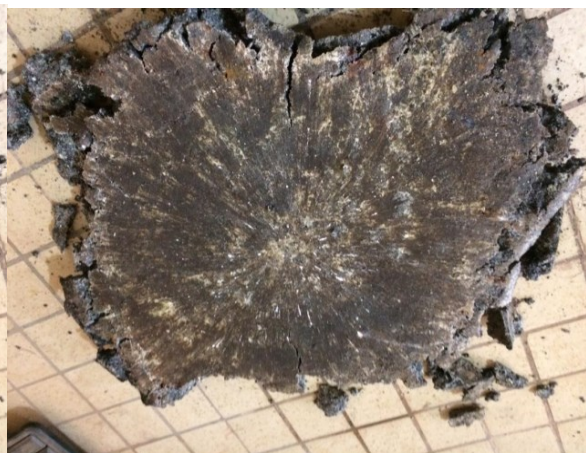
A 3-1: Prototypes of pavers using MPB (interior backyard) and PWC (bearing heavy load) made from plastic wastes before and after demolding
