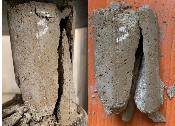
Figure 4-14: Images of typical failure behaviors observed in compressive strength tests on conventional mortar samples
