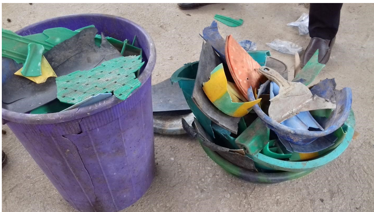
A 1-4: Samples of some a) HDPE and b) LDPE plastic wastes used during the preparation of the MPB and PWC materials.
