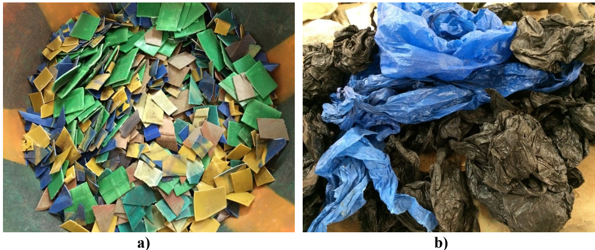
Figure 4-2: Samples of (a) HDPE and (b) LDPE plastics wastes used in testing program
