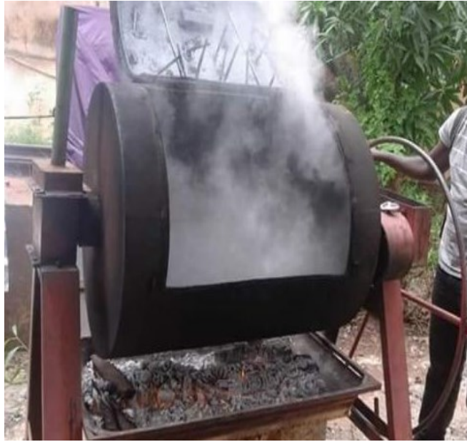
A1-6: Furnace (oven) used for large-scale production of MPB and PWC materials
