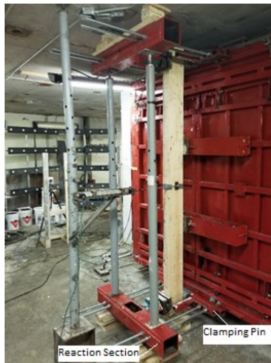
Figure 3.4: Image of experimental setup for glulam, annotated lower components.
