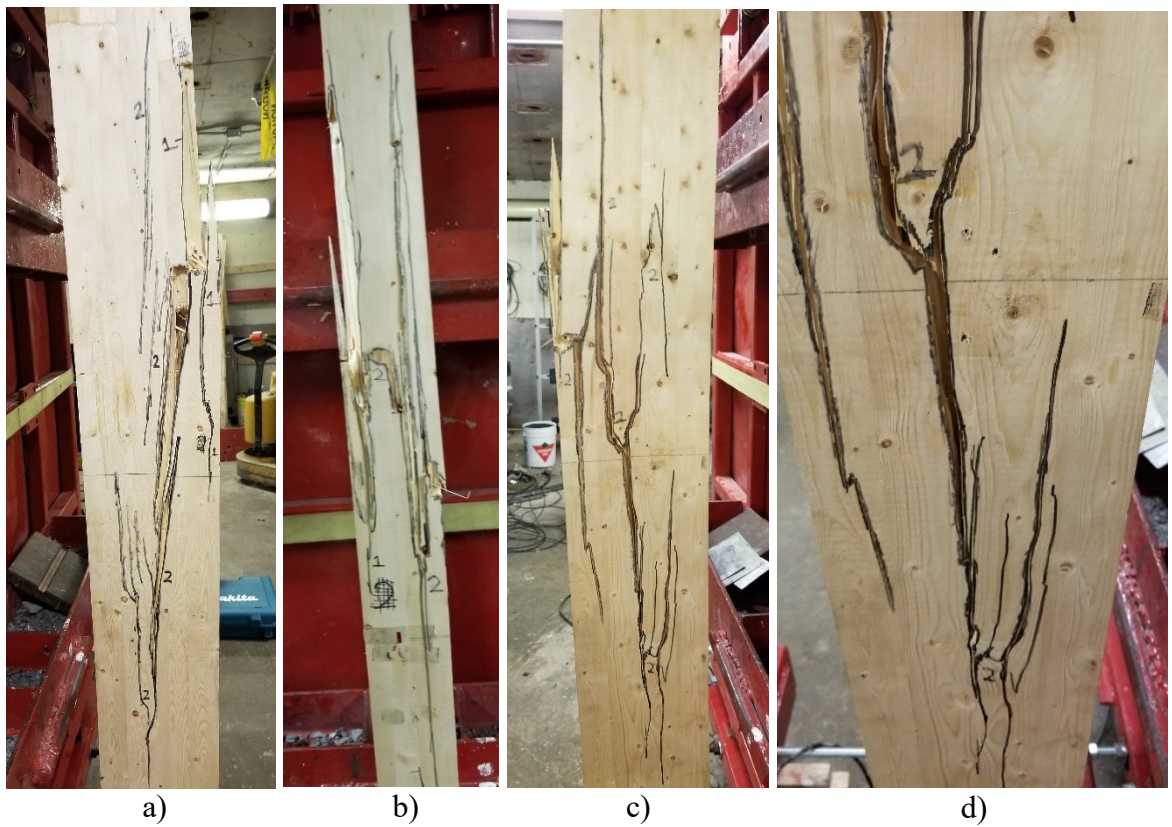
Figure A.18: Final state for shot GL2.2: a) Left side b) Tension face c) Right side d) Reversing crack details
