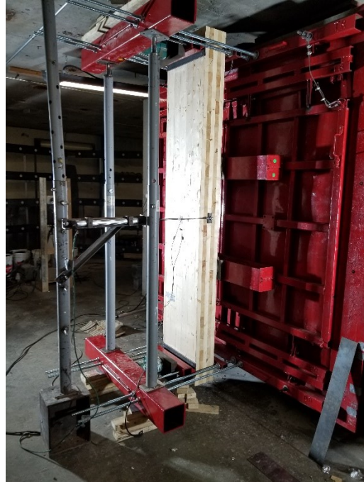
Figure 3.5: Image of experimental setup for CLT
