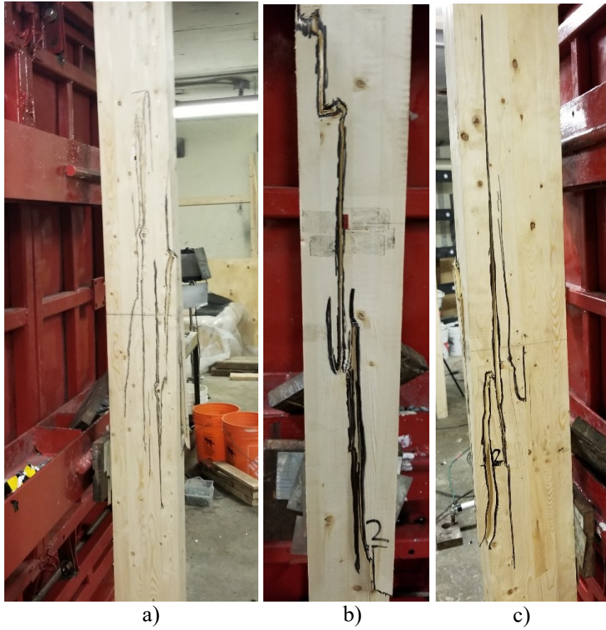
Figure A.36: Failed specimen after test GL3.3: a) Left side b) Tension face c) Right side
