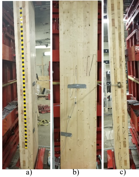
Figure A.54: Specimen after shot CLT2.1: a) Left side b) Tension face c) Right side
