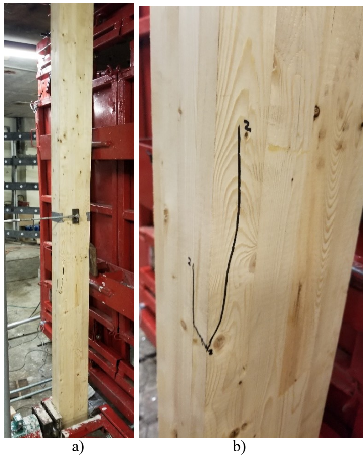
Figure A.31: a) Superficial damage after shot GL3.2 b) Superficial crack detail
