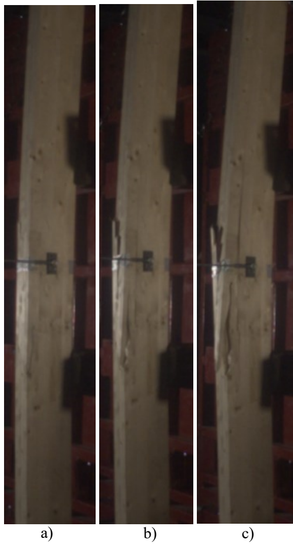
Figure A.37: Progression of failure during test GL3.3: a) 15.5 ms b) 21 ms c) 28 ms
