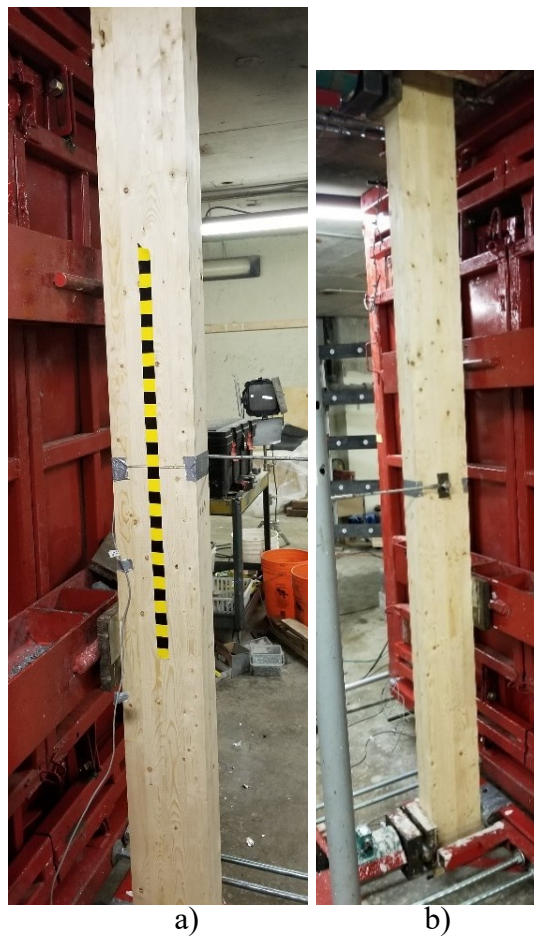
Figure A.25: Undamaged specimen after test GL3.1: a) Left side b) Right side
