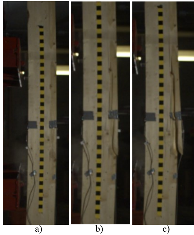
Figure A.6: Progression of failure during test GL1.1: a) 21 ms b) 22.5 ms c) 25.5 ms
