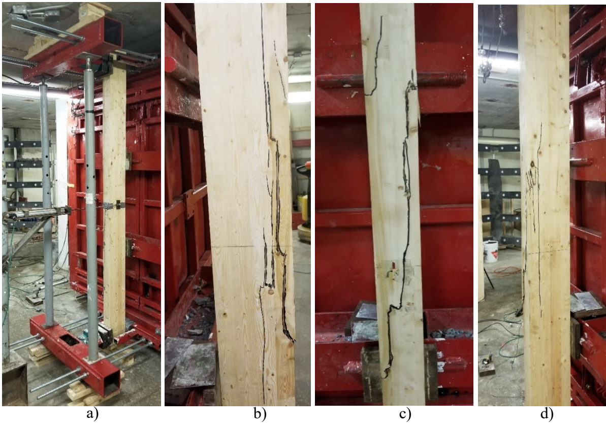
Figure A.5: Initial (a) and failed state (b, left side; c, tension face; d, right side) for test GL1.1
