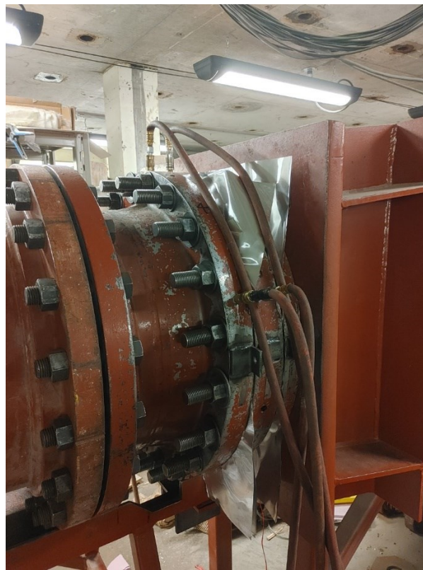
Figure 3.2: Closed diaphragm section, with pressure lines and foils.
