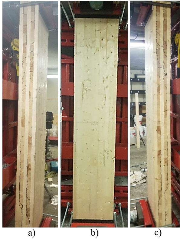
Figure A.82: State of specimen after test CLT3.2: a) Left side b) Tension face c) Right side
