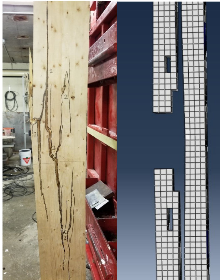
Figure 6.17: Side-by-side comparison between experimental cracking and model deletion for GL2.2
