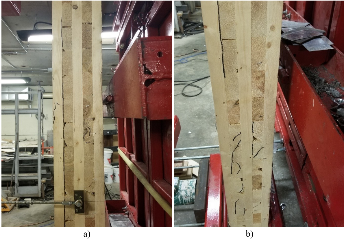
Figure 4.12: a) Vertical crack on right side b) Right side rolling shear cracks
