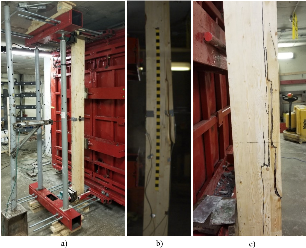
Figure 4.3: a) Specimen GL1 before testing b) Failure during test GL1.1 c) Failure cracks, left side
