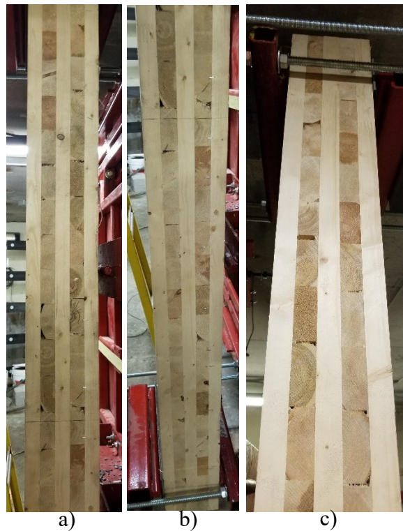
Figure A.53: Pre-existing transverse gaps in specimen CLT2 a) Right side, top b) Right side, bottom c) Left side, top
