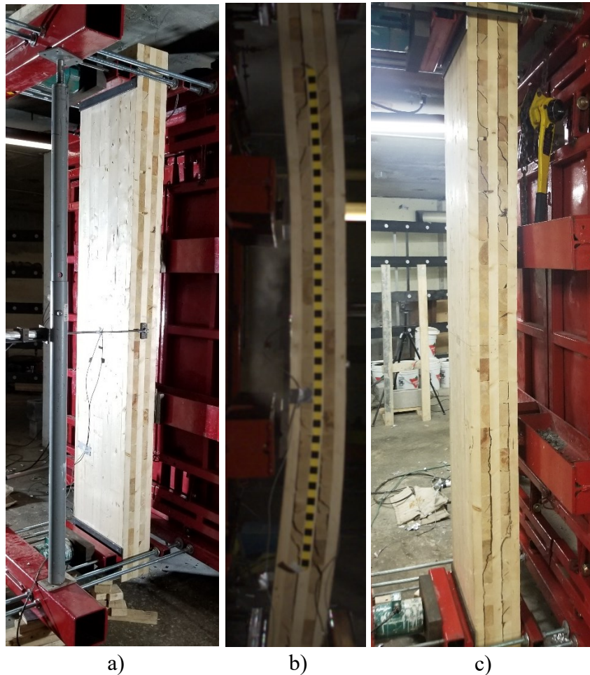
Figure 4.15: a) Undamaged specimen before testing b) Development of rolling shear cracks during test c) Damaged state of panel, right side
