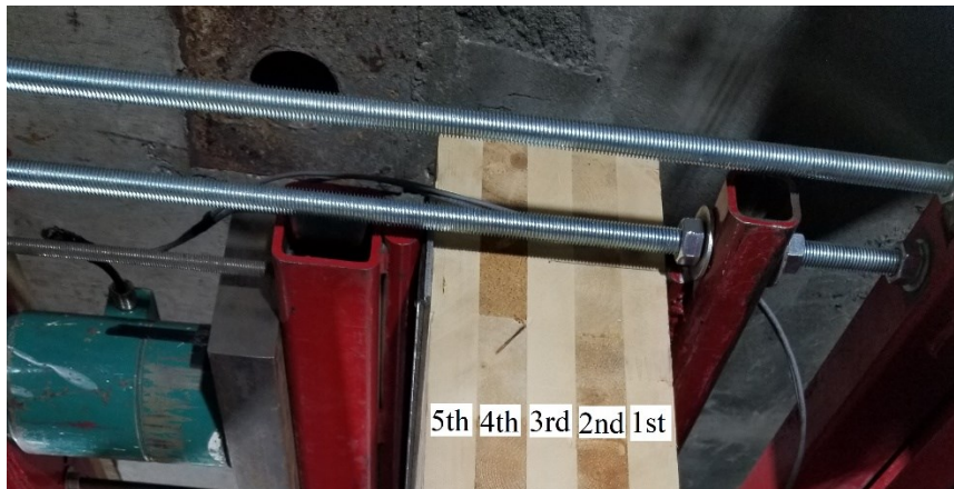
Figure 4.2: CLT specimen end, left side, with annotated ply order
