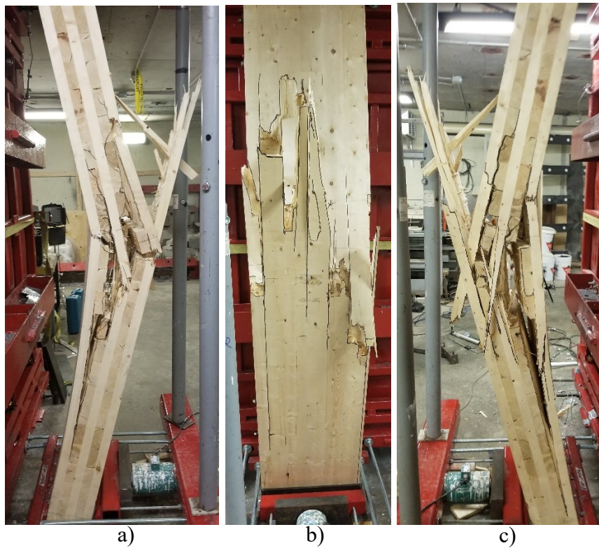
Figure A.43: Overview of final state for shot CLT1.1: a) Left side b) Tension face c) Right side
