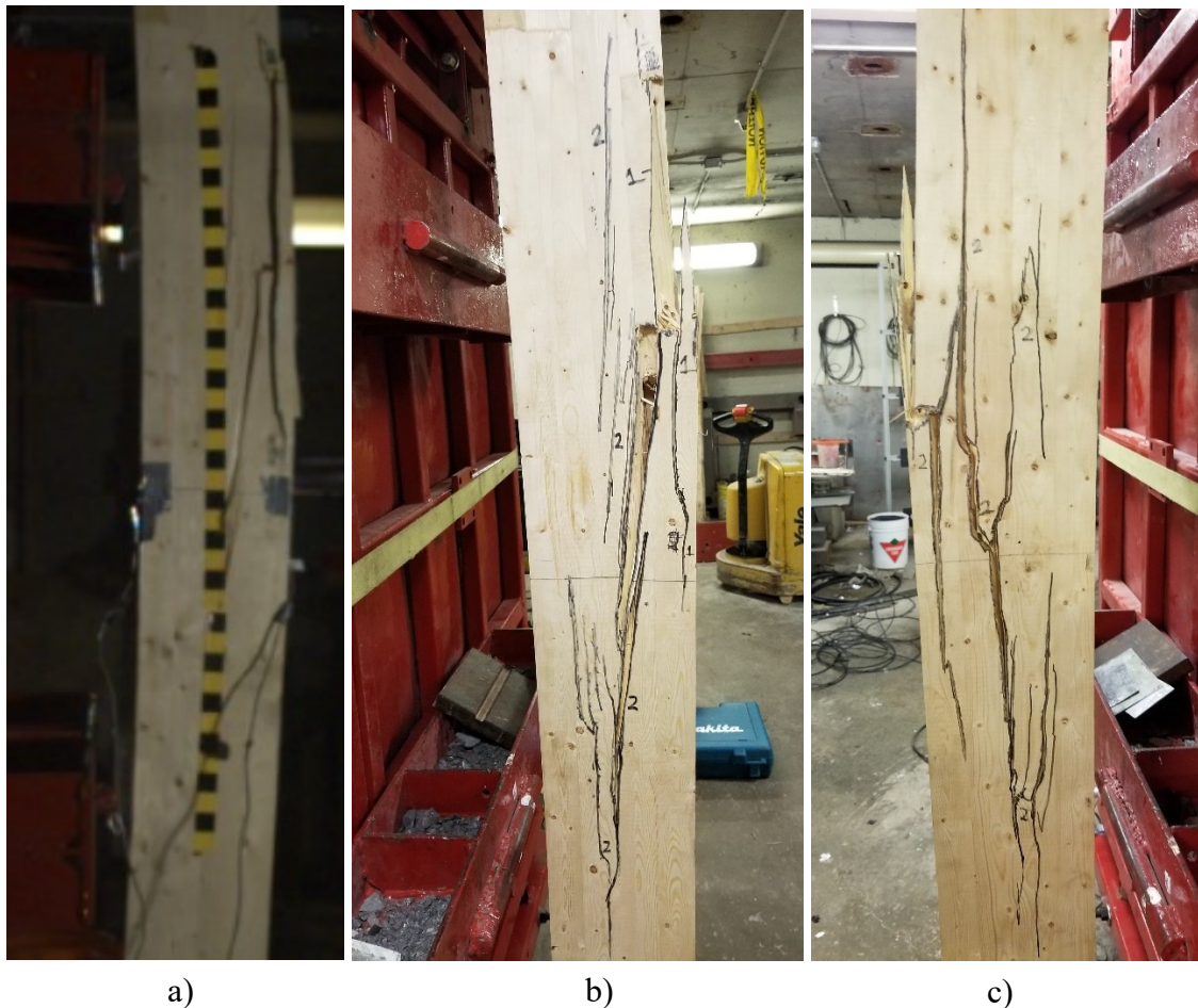
Figure 4.5: a) Initiation cracks during test GL2.2 b) Failure cracks left side c) Failure cracks right side
