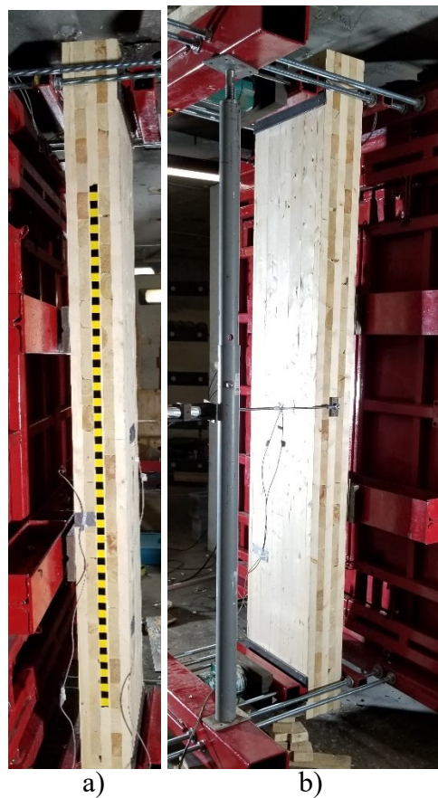
Figure A.76: Undamaged specimen after test CLT3.1: a) Left side b) Right side and tension face
