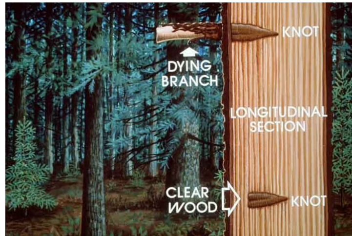
Figure 1.2 Illustration showing knot formation, a type of defect occurring during growth [6]
