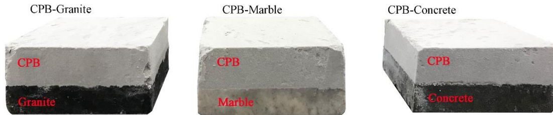
(a) Samples made with different types of rocks (JRC=0, curing for 1 day)
