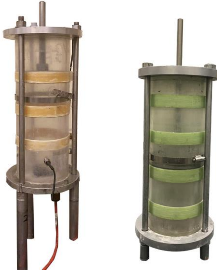
Figure C-7 uOttawa Backfill Curing System (Left one is for monitoring programs, right one is for curing interface sample)
