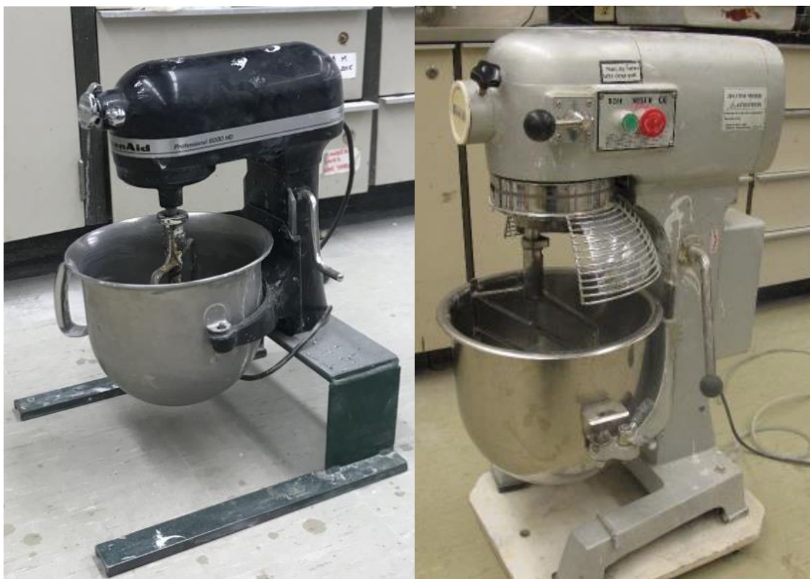
Figure C-5 Mixer for CPB preparation (Left one is for preparing small amount of CPB, right one is for preparing large volume of CPB)
