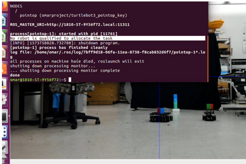
Figure 6.13 The available agents cannot respond to the detected task due to lack of qualification
