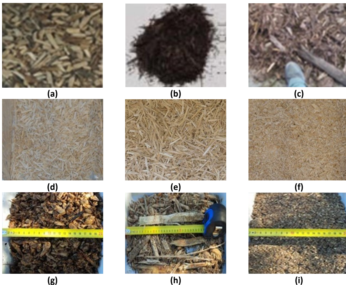
Figure D-1: Forestry, agriculture, & pulp industry biomass residues in various degrees of processing. Forestry residues include (a) willow, (b) torrefied willow, and (c) poplar bark. Agricultural residues include (d) switchgrass stem, (e) switchgrass leaf, and (f) hardwood sawdust. Pulp mill residues include (g) knots, (h) hog, and (i) sludge.
