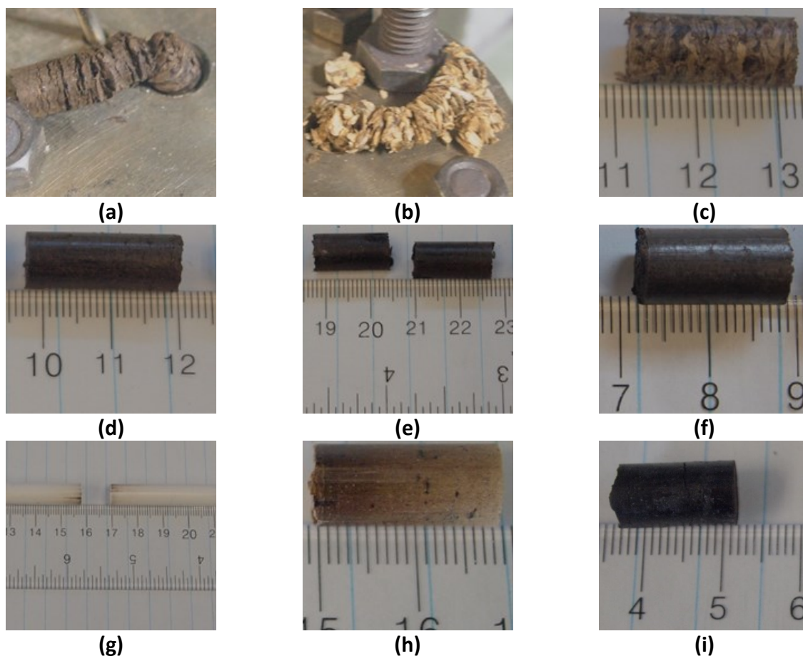
Figure 2-5: Qualitative pellet results for 5 biomass materials (woody, agricultural, pulp, and cellulose). (a) Pelletization for wet torrefied willow at 90°C; (b) untreated willow pelletization tested the same as in (a); (c) untreated willow with 2 wt% moisture at 200°C; (d) torrefied willow pellets produced the same as (c); (e) two switchgrass stem pellets at 300°C; (f) sludge pulp residue at 300°C; and pure cellulose produced (g)-(i) at 80, 250, and 300°C respectively. All pellets presented produced at 215 MPa. Additional qualitative results available in Figure D-2.
