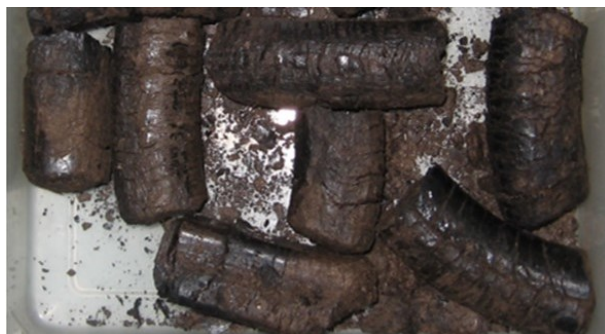
Figure 2-15: Commercial torrefied briquettes and the resulting fines after a 48-hour immersion.
