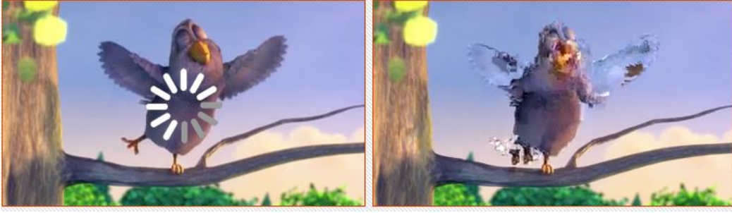
Fig. 2.1 Freezing in TCP and error artifacts in UDP
