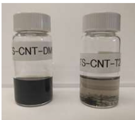
Figure 4.6 Tip sonicated CNTs in DMF and Milli-Q water before adding helicase. Samples in DMF retained higher concentration of CNTs, and the solution appeared darker in color.
