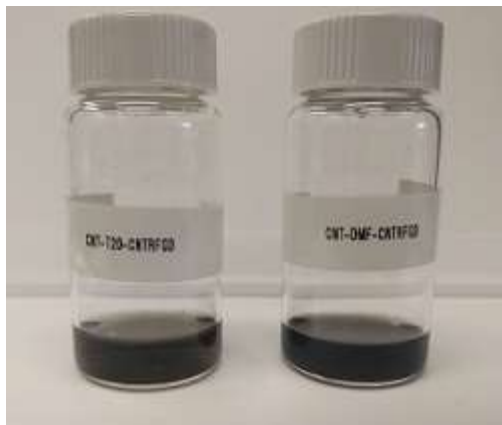
Figure 4.2 CNTs in Milli-Q water (left) and DMF (right) after bath sonication
