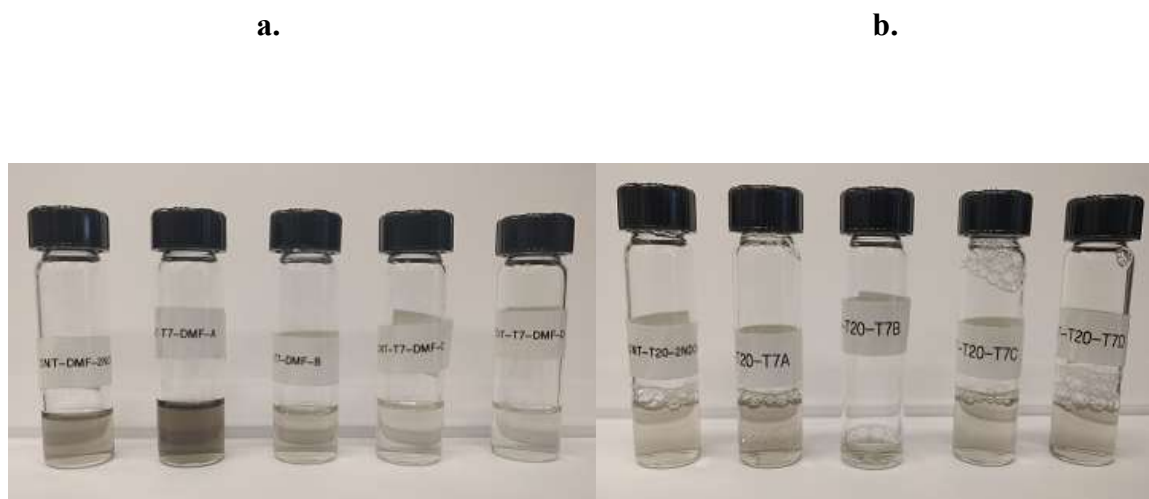
Figure 4.4 CNTs in (a) DMF and (b) Milli-Q water centrifuged after helicase incubation. Decreased enzyme concentrations from left to right (from 0 to 0.8 ug/mL).
