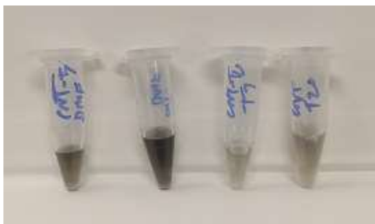
Figure 4.3 CNTs in DMF and Milli-Q before and after helicase attachment (left to right)
