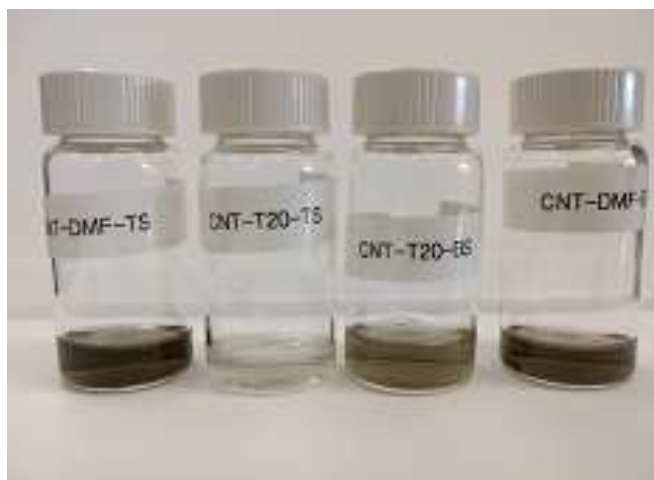
Figure 4.7 Tip sonicated CNTs in DMF and Milli-Q water and bath sonicated samples after helicase incubation and centrifugation
