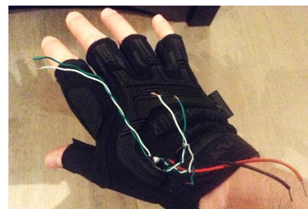
Figure 3-12. Embedding the actuators between the fabric layers of the glove.
