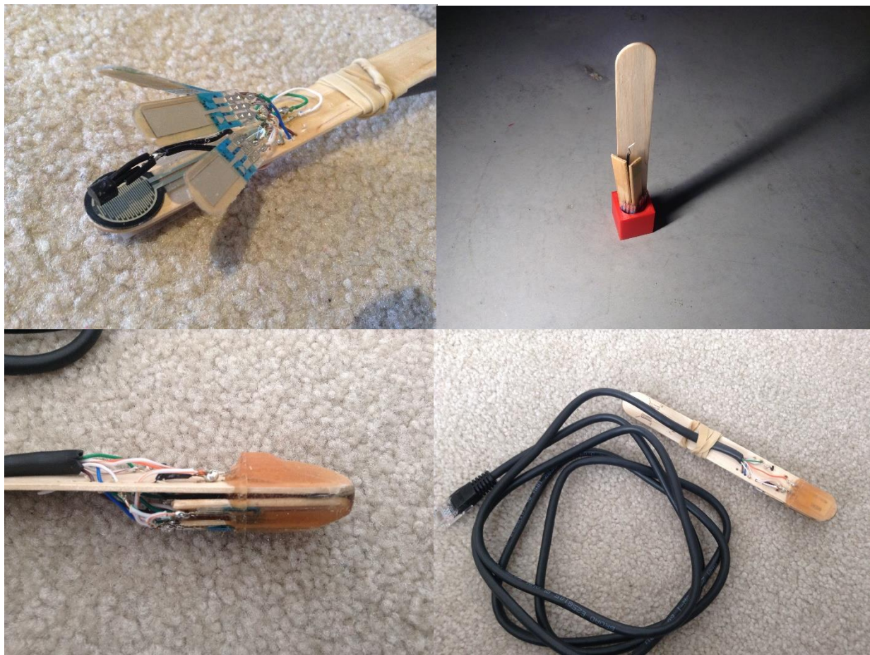
Figure 3-18. Production steps for creation of the initial artificial fingertip with embedded sensors and rubber casing. 6 sensors were attached to the wooden craft stick (top left), then inverted into a mold in which the rubber compound was poured and left to cure overnight (top right), finished product ready for use by connecting 45cm long, CAT-5 cable to the circuit board sensor input port (bottom left & right).
