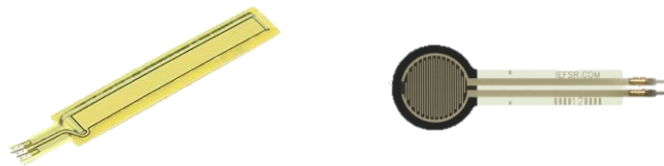
Figure 3-4. Thin potentiometer (left) and a Force Sensing Resistor (right) two mechanical force sensors used for artificial
