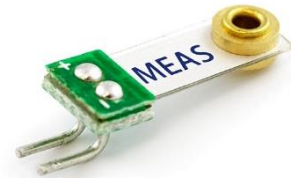
Figure 3-5. Piezoelectric vibration sensor used in the prototype sensor array.
