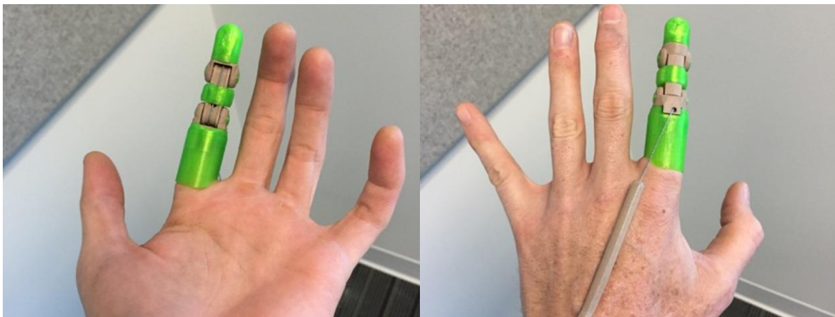
Figure 3-3. The Knick Finger: A mechanically-controlled, 3D-printed prosthetic finger, Courtesy of [77].
