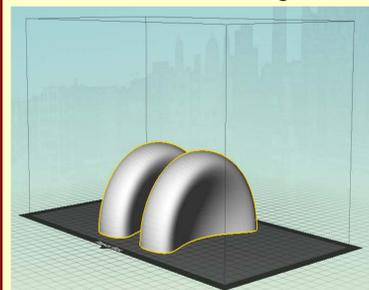
Fig.4: RBC split into two halves seen in the Makerbot® software
