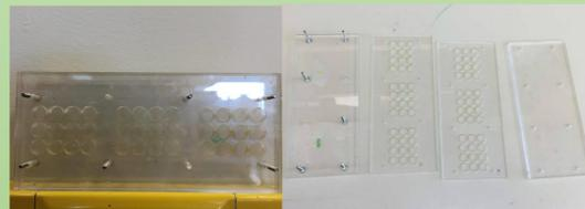
**Figure 4. Two-layered chamber for mating behaviour assay.** Picture showing the two-layered chamber used for mating behaviour assay. One chamber contains 36 holes in which the female and male flies were added to during assay. Females were added to bottom layer and then a plastic divider was added to separate them from males. Males were then added to the top layer and enclosed within the chamber using a hard plastic cover.
