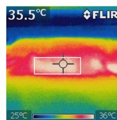
Figure 4. IR image of heat signature of 40W IR bulb on PDMS chip set 5 cm above
