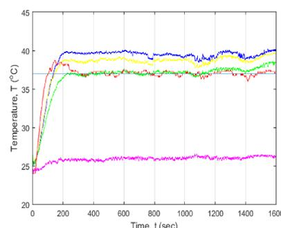
Figure 5. 50W IR bulb, 5 cm above the chip and the FBC is located at position 2. Overshooting is observed for the controller.
