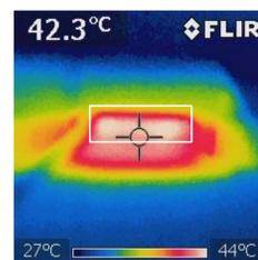
Figure 6. IR image of heat signature of 50W IR bulb on PDMS chip set 5 cm above
