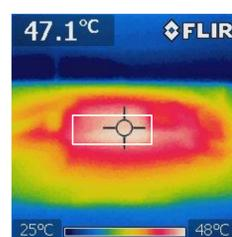
Figure 8. IR image of heat signature of 50W CER bulb on PDMS chip set 5 cm above
