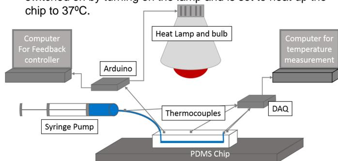
Figure 1. Overview of touchless heating system
