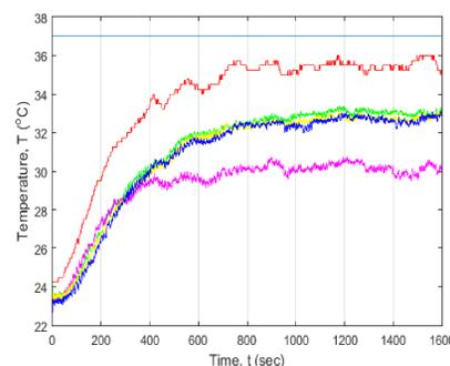
Figure 3. 40W IR bulb, 5 cm above the chip and the FBC is located at position 2. The desired temperature is not reached for the average chip temperature.
