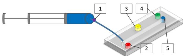
Figure 2. Location of the thermocouples position and corresponds to the colors on the graph. Position 5 is immersed in the fluid.
