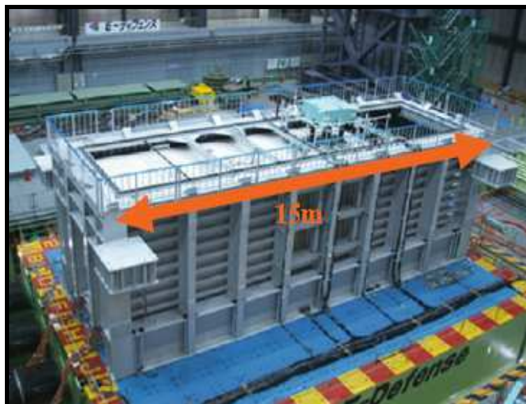
Figure 6.7 E-Defense large shaking model test on lateral flow of liquefied sand induced by failure of sheet-pile quay wall (Motamed et al., 2009)
