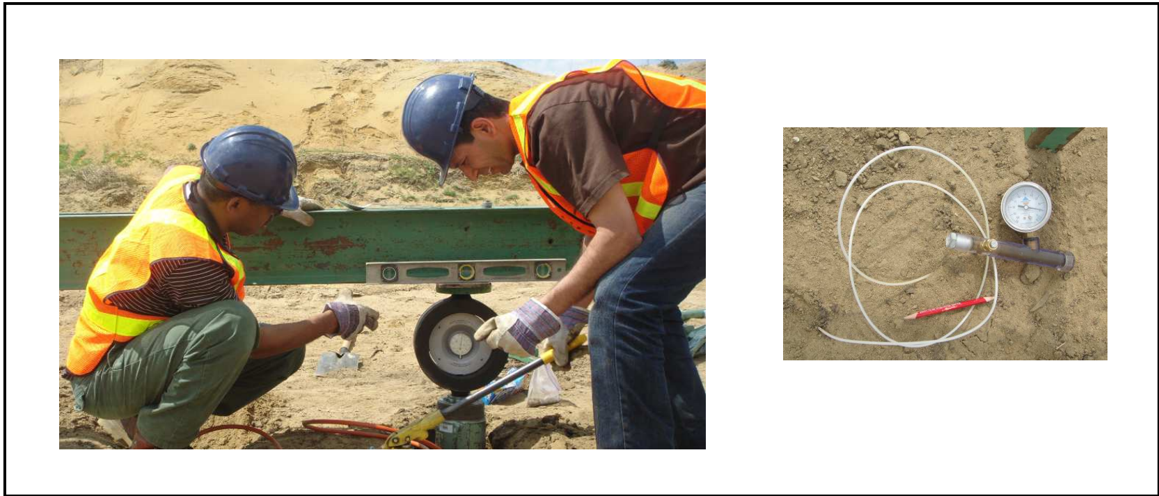
Figure 4.5 Photos of the PLT setup and a Tensiometer used at the site
