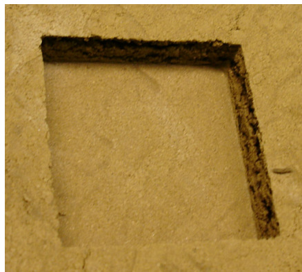
Figure 3.19 Indentation from model footing tests.
