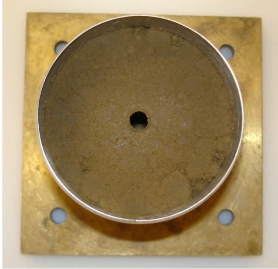
Figure 2.24 A cylindrical aperture in a compacted soil specimen to insert the ceramic cup of the conventional tensiometer.
