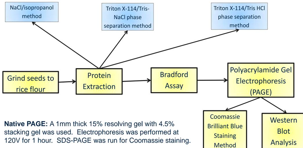
**Native PAGE:** A 1mm thick 15% resolving gel with 4.5% stacking gel was used. Electrophoresis was performed at 120V for 1 hour. SDS-PAGE was run for Coomassie staining.
