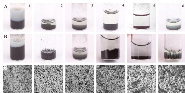
**Figure 1.** Six syntheses of nickel nanoparticles (NNP) produced under varying conditions of  $[\text{Ni}(\text{OH})_2]$ ,  $[\text{PVP}]$ , pH, and reaction time. Row A displays NNP without influence of a magnet. Row B shows the influence of NNP under the presence of a magnet. Row C contains pictures of SEM at 40 000 magnification.
