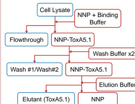
**Figure 2.** Flow chart of one cycle of the protein purification process. This cycle is repeated three times throughout the protocol. Supernatants (in blue) are analyzed by SDS-PAGE.
