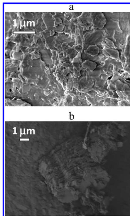
**Figure 5.** SEM images of the aggregated microcomposite obtained by reaction of DMSO-K with (a) IL\_1 (9000 $\times$  magnification) and (b) IL\_2 (20 000 $\times$  magnification).
