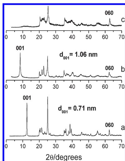
**Figure 1.** Powder XRD patterns ( $2\theta = 2\text{--}70^\circ$ ) of (a) kaolinite; (b) Urea-K, and (c) the exfoliated nanocomposite obtained after reaction of Urea-K with IL\_1.
