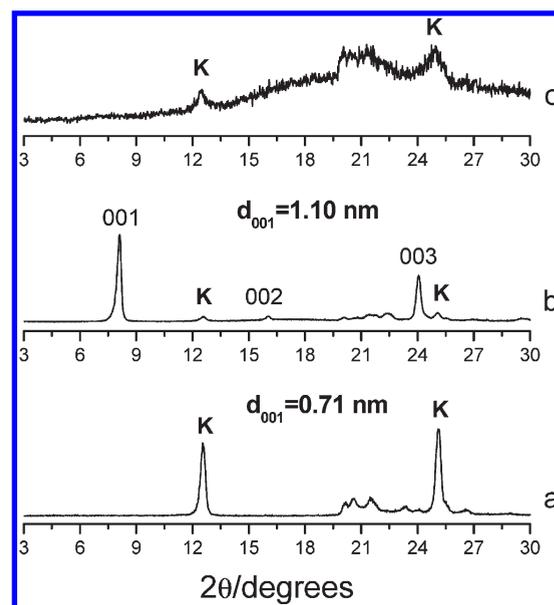
**Figure 2.** Oriented XRD patterns ( $2\theta = 3\text{--}30^\circ$ ) of (a) kaolinite; (b) DMSO-K, and (c) the resulting microcomposite obtained after reaction of DMSO-K with IL\_1.
