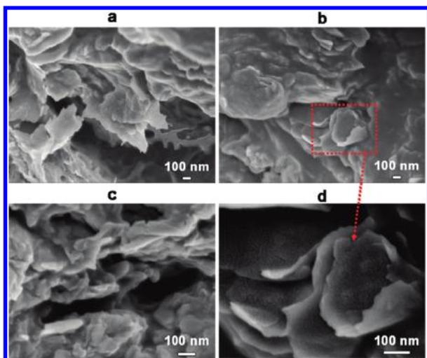
**Figure 4.** SEM images of the exfoliated nanocomposite obtained by reaction of Urea-K with IL\_1: (a,b) 50 000 $\times$  magnification, (c) 100 000 $\times$  magnification, and (d) 140 000 $\times$  magnification.
