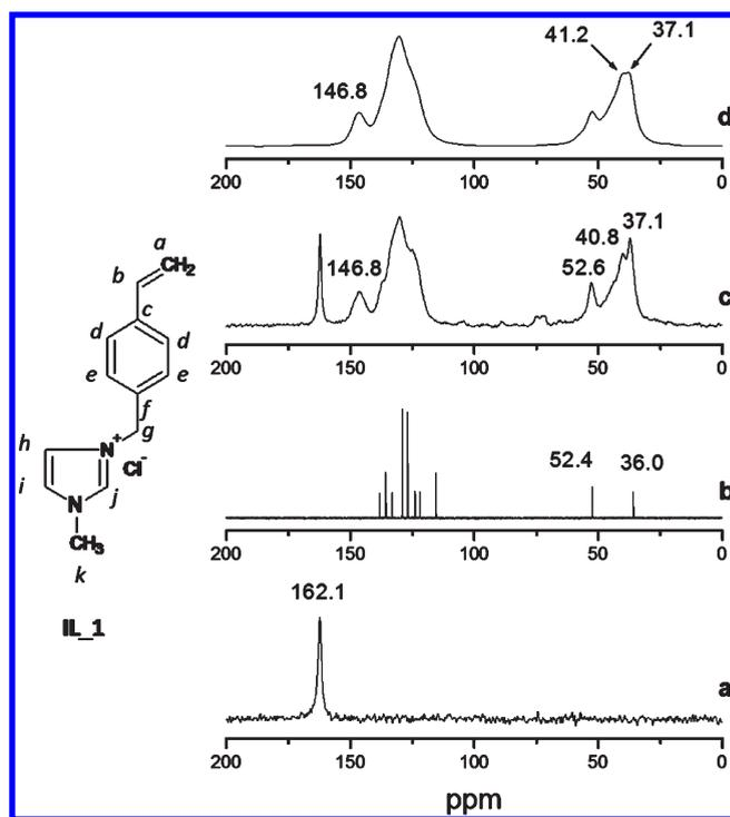
**Figure 3.** Solid-state  $^{13}\text{C}$  CP/MAS NMR spectra of (a) urea-K intercalate; (b)  $^{13}\text{C}$  NMR spectrum of IL\_1 in solution, given for reference; (c) the resulting exfoliated nanocomposite obtained after the reaction of Urea-K with IL\_1; (d) the polymer obtained by polymerization of IL\_1.
