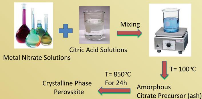
Fig. 2. Process of creating perovskites via the sol gel method.
