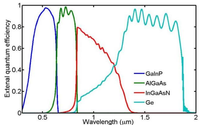
Fig. 1: External quantum efficiency curves for each subcell in a lattice-matched 4JSC.
