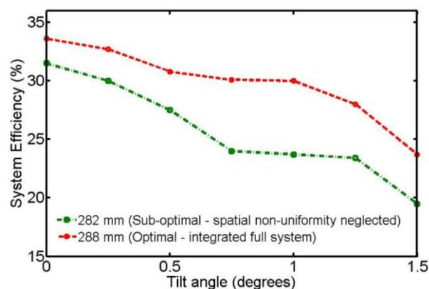
Fig. 5: Overall efficiency as a function of tilt angle with the sub-optimal and optimal working distances.
