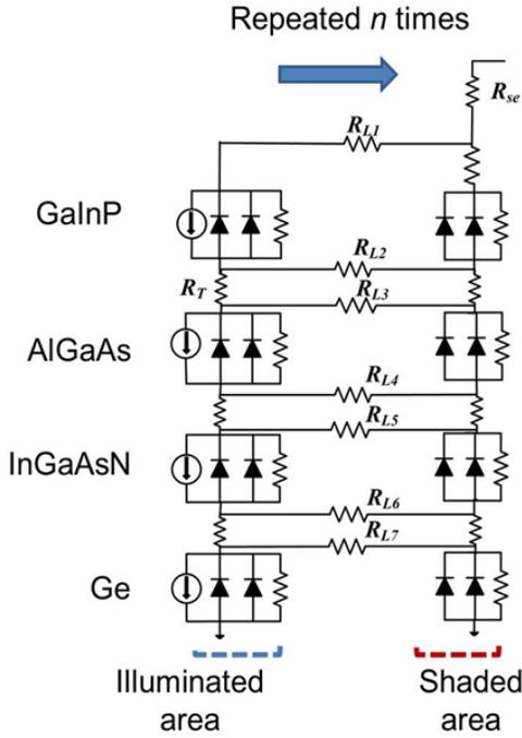
Fig. 2: A functional block in a 2-D distributed equivalent circuit model for a four junction solar cell. A functional block is repeated  $n$  times to generate the model of a complete 4JSC in SPICE.
