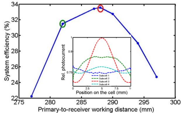
Fig. 4: Overall system efficiency as a function of primary-to-receiver working distance including the effects of spatial and spectral non-uniformities. Efficiencies at a working distance of 282 mm (obtained ignoring spatial non-uniformity) and 288 mm (obtained using integrated optimization) are highlighted. Inset shows the relative photocurrent distribution as a function of cell position for each subcell at the optimal working distance of 288 mm.
