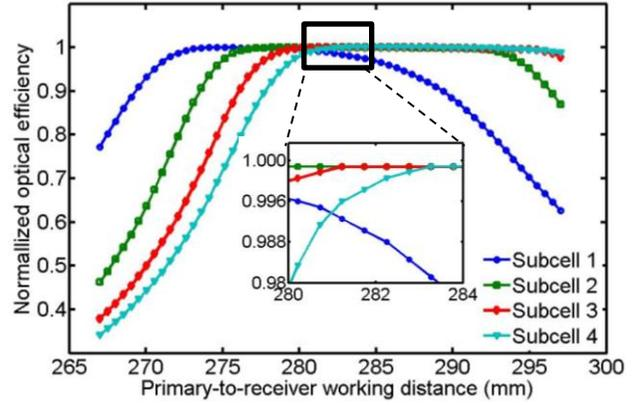
Fig. 3: Normalized optical efficiency relative to each subcell as a function of primary-to-receiver working distance. The zone within which the normalized efficiency for all subcells is greater than 98% is highlighted. Inset shows the enlarged view of the optimal zone.
