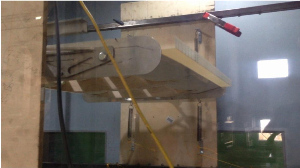
Figure 3.1.24 Setup for the dynamic test in the wind tunnel
