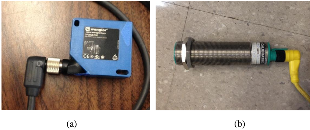
Figure 3.3.1 (a) Laser sensor and (b) ultrasonic sensor used in the dynamic test
