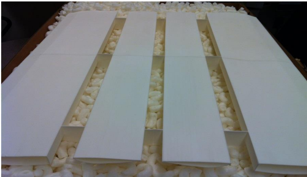
Figure 3.1.10 3D-printing model of the four individual bridge deck shells
