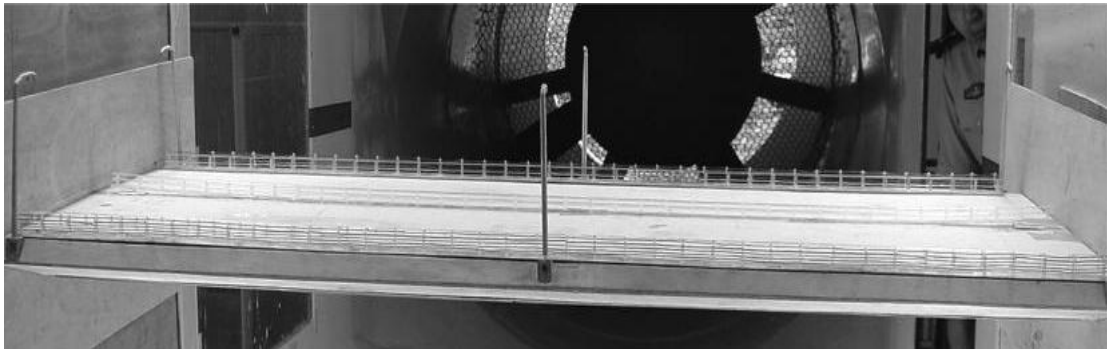
Figure 2.3.15 Wind tunnel testing of a twin-deck sectional model [79]
