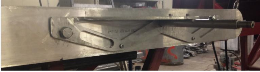
Figure 3.1.16 Elliptical aluminum end plate with connecting frame
