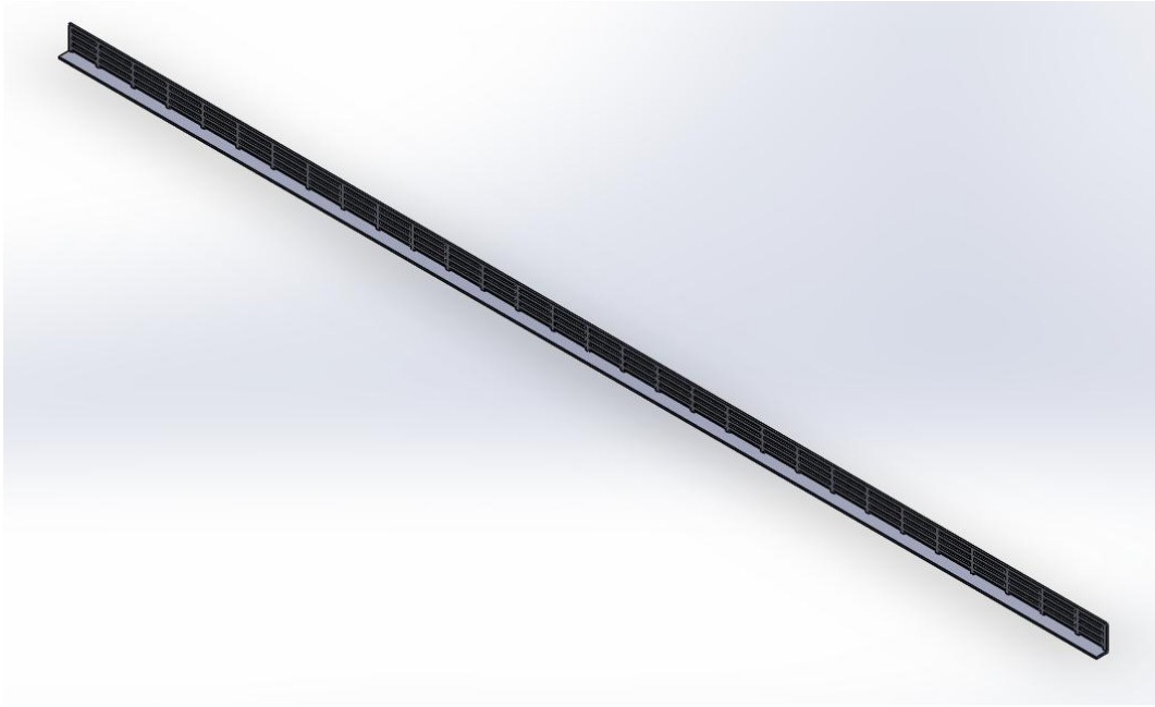
Figure 3.1.7 SolidWorks model of the windshield barrier with 20 mm height
