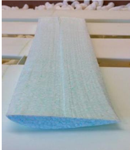
Figure 3.1.13 Solid low density foam core used for inside of the four individual bridge deck shells
